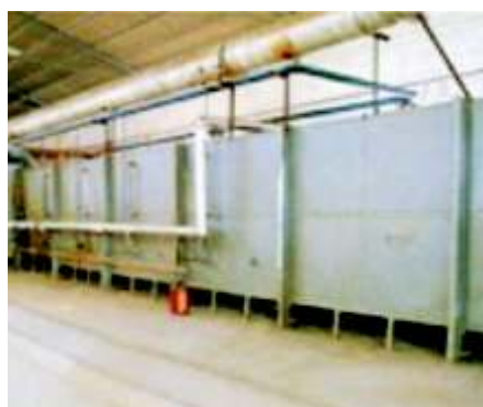
Tunnel Furnace (1550°C)
