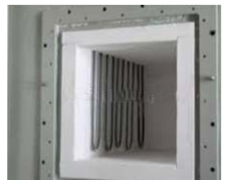
Lab Muffle Furnace (1700°C)
